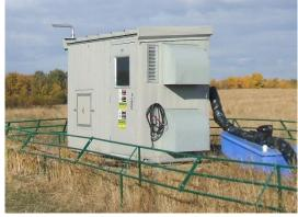
Gas Pro specializes in the packaging of dependable, quiet, single well gas compressors for low pressure wells.
